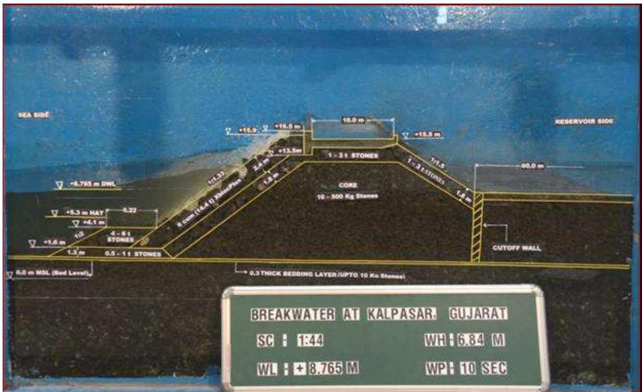
Photo 11 : Wave action on the armour of breakwater cross-section at 0.0 m bed level during breaking wave height ( H_s ) of 6.84 m at Design Water Level (DWL) of +8.765 m
