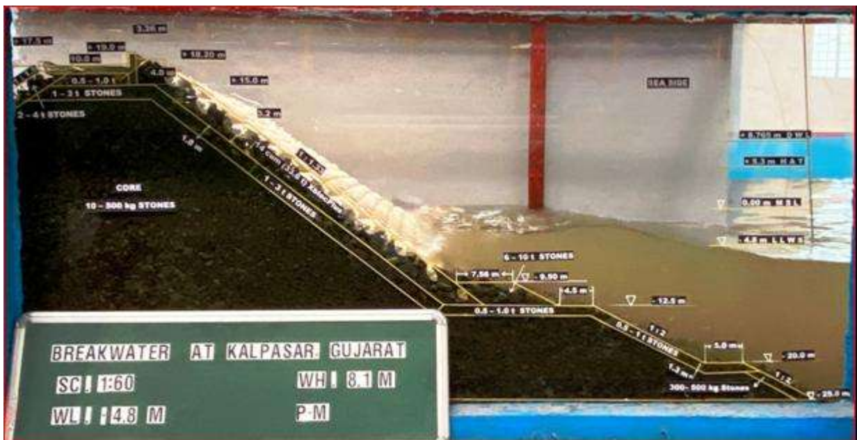
Photo 9 : Wave action on the armour of breakwater cross-section at -25.0 m bed level during significant wave height ( H_s ) of 8.1 m at Lowest Low Water Level (LLWL) of -4.8 m
